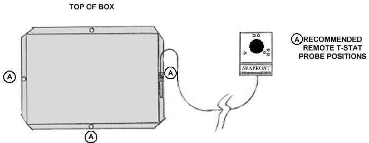
The SEA FROST BD thermostat is variable. Turning the knob fully counterclockwise turns the unit "OFF". The fully clockwise setting is the coldest (three snowflakes). The thermostat may be adjusted to obtain any temperature desired in the cabinet. The thermostat may be calibrated should the warmest setting be too cold. To calibrate the thermostat remove the mounting screws and tip the panel forward. Remove the electrical tape to expose a black torx adjustment screw about an inch into the case.
