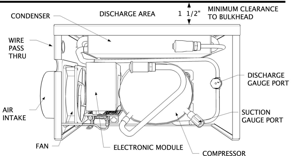
An un-ducted unit in a poorly ventilated small space will heat the air, lowering the cooling capacity and possibly causing damage by overheating the compressor.
